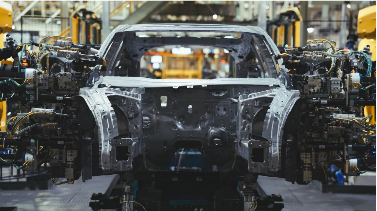
Robot assembling door panels to the AFEELA 1 body-in-white on the production line.
