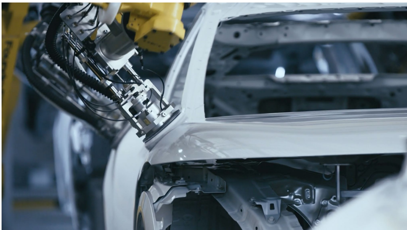
A newly introduced robot polishing the AFEELA 1 for paint undercoat preparation.
